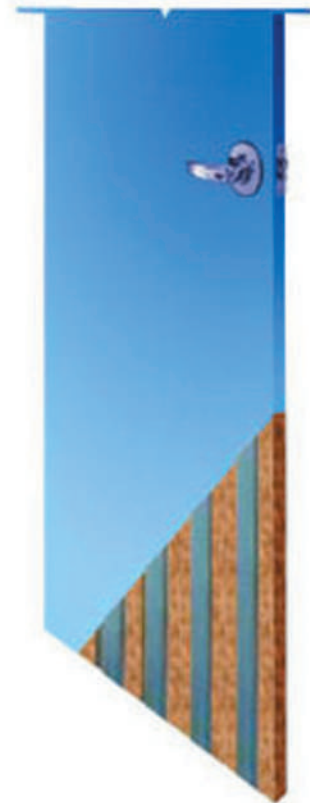
STEEL STIFFENED WITH ROCK WOOL
